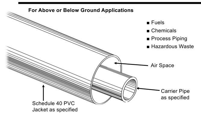
Rovanco's Containment PVC Quick Fit System is designed for piping systems above or below ground. A High-quality, durable PVC jacket, provides an economical system.
